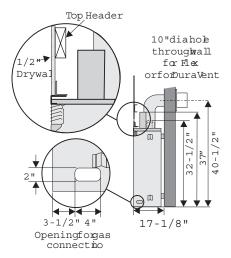
Note: 40-1/2" (1029mm) is the minimum height for both flex termination or Simpson Dura-Vent venting.
